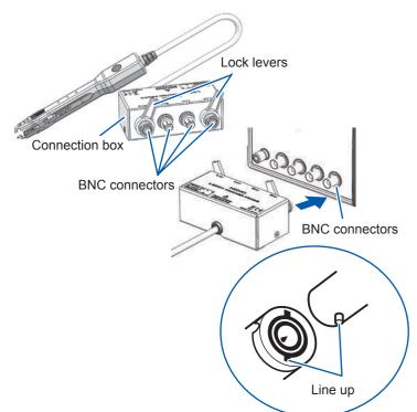
2 Twist the lock levers to secure the connection box to the measuring instrument.
