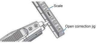
**3** Perform correction with the measuring instrument.
