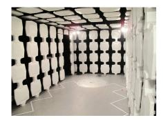
The SpaceSaver™ 26H is an RF-shielded semianechoic chamber providing a multi-purpose environment for radiated immunity and precompliant emission testing. This compact chamber provides an anechoic test environment that supports testing up to 40 GHz with anechoic performance equal to or better than that required for radiated immunity testing per most standards including IEC, pre-compliant emission testing, and design and debugging applications.
